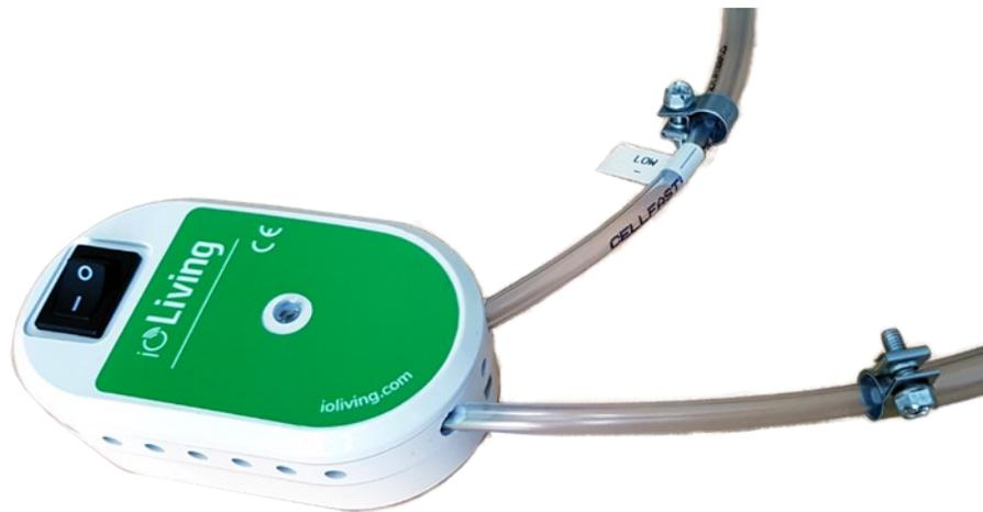
Data collector with Swiss SDP37 precision sensor that measures pressure difference and room air temperature and humidity.
