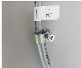
When installing the conducting hose to a building, it must be sealed with a tape or a Blu-Tack. The measurement itself must not affect to the pressure difference under the measurement.
